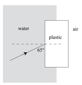
(b) The ray of light deviates (or changes direction) through an angle of 4.0° as it enters the plastic. The refractive index of plastic is 1.5.
